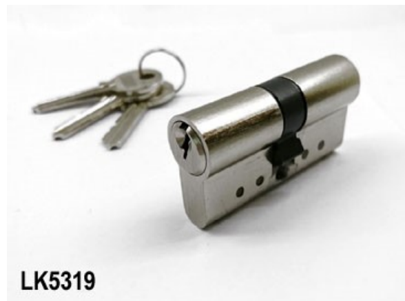
LK5319 Brass Profile Cylinder with 3 keys, 5 pins each side with anti-bump, anti-drill, anti-snap, anti-pick and s/s bar bridge
